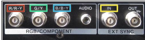
An example of RGBS (and component YPbPr) video input BNC jacks on the back of a Sony PVM monitor.
